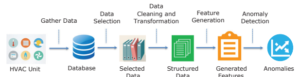
Fig. 3. A standard workflow of applying anomaly detection approach on HVAC data.
