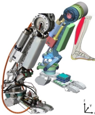
Fig. 2 Lower leg - ankle joint - foot - assembly: Next to the biological inspiration (in the back), the CAD-model (middle) depicts the developed lower leg structure, whereas a photograph of the lower leg and ankle joint with the foot is shown in the front.
