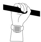
**Figure 1:** Smartwatch concept with two displays – one on each side of the user's arm. Depending on the arm's orientation, the content can be shifted between the displays: when doing pull-ups for example, the inner display can still be seen while the outer one is not in the user's field of view. sued, e.g. pull-ups. To get rid of this limitation, a device with two displays (one on each side of the arm, see Figure 1) or even more (such as e.g. [21]) could be used.
