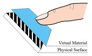
**Figure 1:** The concept of augmenting texture perception by overlaying a physical structure with a virtual texture, where the physical structure is created by a 3D printer.
