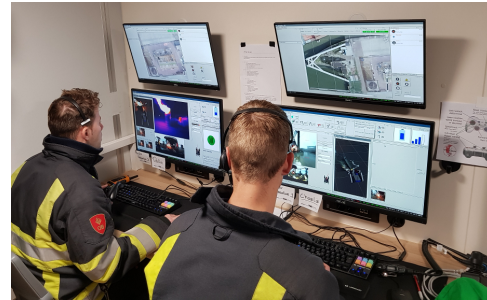
Figure 2: Responders operating the UGVs using the OCU (bottom) and tactical map (top).
